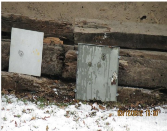
Left: The shot through; concrete panel 55mm
